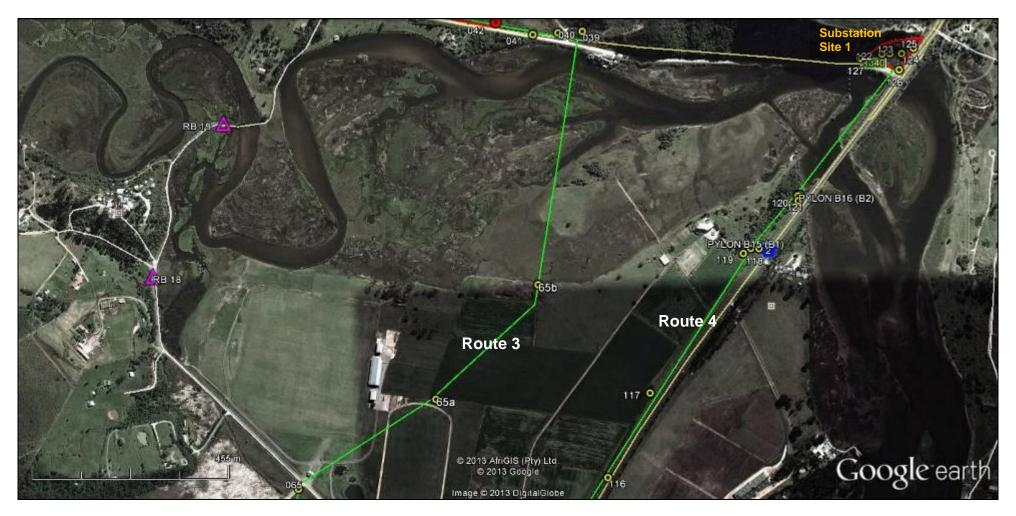
**Figure 11.** Google Earth<sup>TM</sup> aerial image showing the proposed 66kV powerline Route 3 and Route 4 (green lines) and Substation Sites 3 (red lines) between placemark 69a to waypoint 065. The numbered yellow circle icons are the waypoints from the 2013 survey whereas the numbered purple triangle icons are form McDonald's (2007) survey. The numbered icons 69a and 67b are placemark points, i.e. not field samples but used to designate key features in the landscape.
