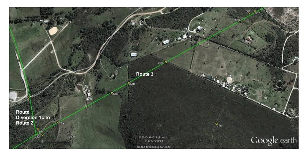
**Figure 9.** Google Earth<sup>TM</sup> aerial image showing the proposed 66kV powerline route 3 (green lines) between waypoints 033 to 067. The numbered yellow circle icons are the waypoints from the 2013 survey. The numbered icons 33a and 33b are placemark points, i.e. not field samples but used to designate key features in the landscape.
