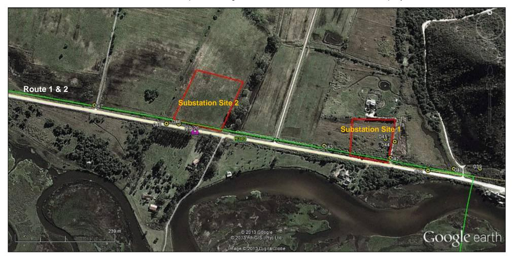
**Figure 19.** Google Earth<sup>TM</sup> aerial image showing the proposed 66kV powerline Route 1 & 2 (green lines) between waypoint 040 and placemarks 047, including proposed Substation Site 1 and 2. The numbered yellow circle icons are the waypoints from the 2013 survey.
