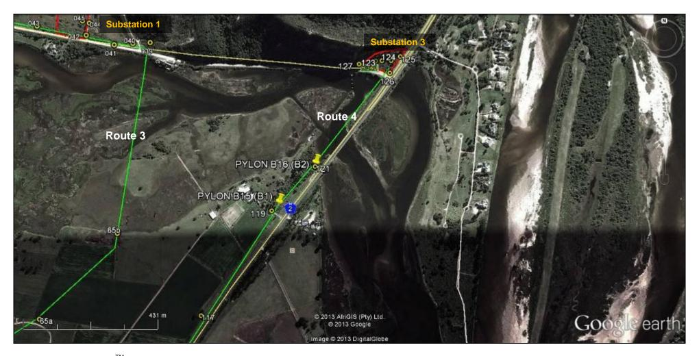
**Figure 24.** Google Earth<sup>™</sup> aerial image showing the proposed 66kV powerline Route 4, Route 3 (green lines) and Substation Sites 2 & 3 between waypoint 117 and placemarks 126 and proposed Substation Site 3. The numbered yellow circle icons are the waypoints from the 2013 survey.
