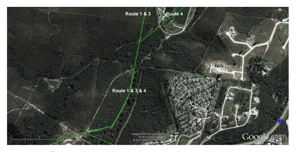
**Figure 6b.** Google Earth<sup>™</sup> aerial image showing the proposed 66kV powerline Routes 1 & 3 & 4 and Route 4 diversion towards the N2 National Highway (green lines) between waypoints 131 to 097. The numbered yellow circle icons are the waypoints from the 2013 survey.
