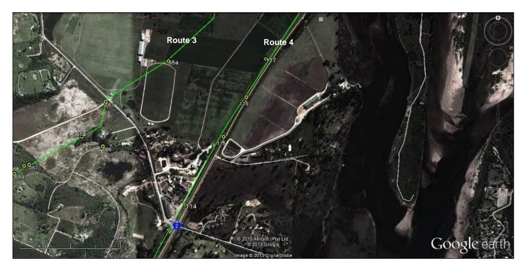
**Figure 23.** Google Earth<sup>TM</sup> aerial image showing the proposed 66kV powerline Route 4 and Route 3 (green lines) between waypoint 114 and placemarks 117. The numbered yellow circle icons are the waypoints from the 2013 survey.
