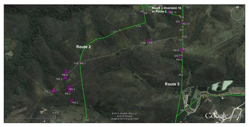
**Figure 14.** Google Earth<sup>TM</sup> aerial image showing the proposed 66kV powerline Route 2 and Route 3 (green lines) between waypoint 083 and 061. The numbered yellow circle icons are the waypoints from the 2013 survey. The numbered purple numbered icons with the 'RB' prefix are McDonald's (2007) sample waypoints.
