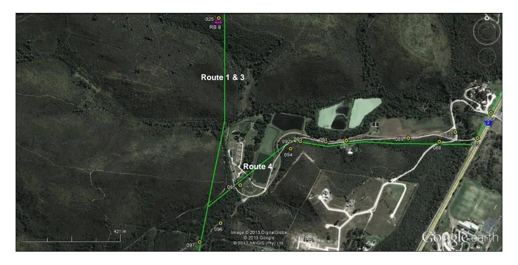
**Figure 7.** Google Earth<sup>™</sup> aerial image showing the proposed 66kV powerline routes 1, 3 & 4 (green lines) between waypoints 097 to 025. The numbered yellow circle icons are the waypoints from the 2013 survey whereas the numbered purple triangle icons are form McDonalds 2007 survey.
