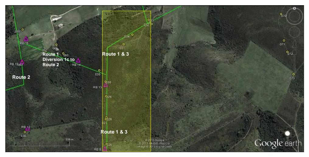
**Figure 8.** Google Earth<sup>TM</sup> aerial image showing the proposed 66kV powerline Routes 1 & 3, Route 2 and Route Diversion 1c to Route 2 (green lines) between waypoints 026 to 033 (yellow shading). The numbered yellow circle icons are the waypoints from the 2013 survey whereas the numbered purple triangle icons are form McDonalds (2007) survey.
