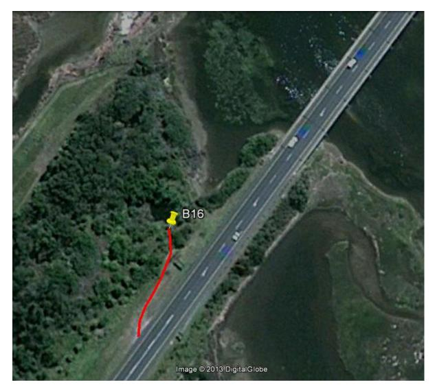
Figure 9. Proposed route of construction track to pylon B16 that should be followed to minimise habitat destruction.
