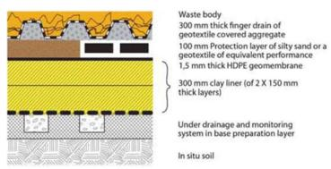
Figure 4-1: Class C landfill barrier system (DEA, 2013b)
