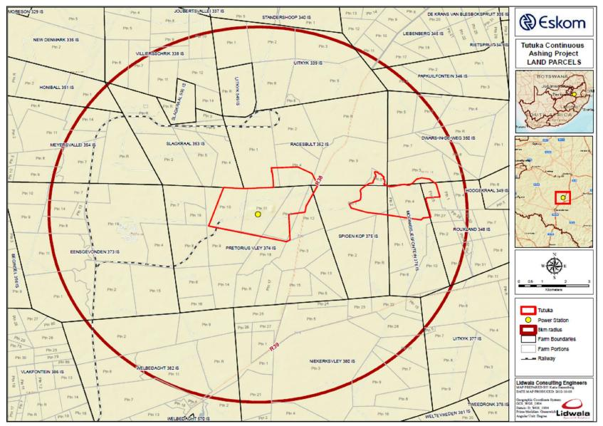
Figure 1. The greater study area for the proposed continuous disposal of ash at the Tutuka Power Station.
