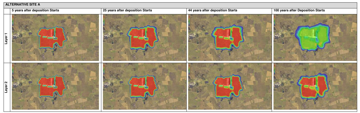
FIGURE 3.4: PLUME DEVELOPMENT FOR ALTERNATIVE ASH DISPOSAL FACILITY SITE A
