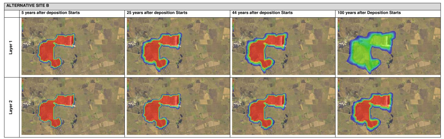
FIGURE 3.5: PLUME DEVELOPMENT FOR ALTERNATIVE ASH DISPOSAL FACILITY SITE B
