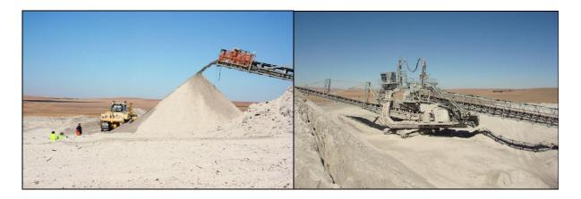
Figure 1: Stacker being used to dispose of ash at the Tutuka Power Station
