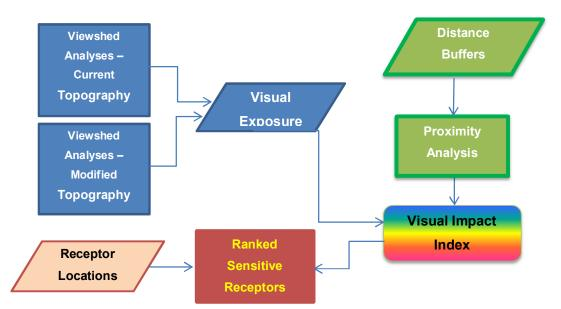
Diagram 1: Preparation process of the Visual Impact Index
