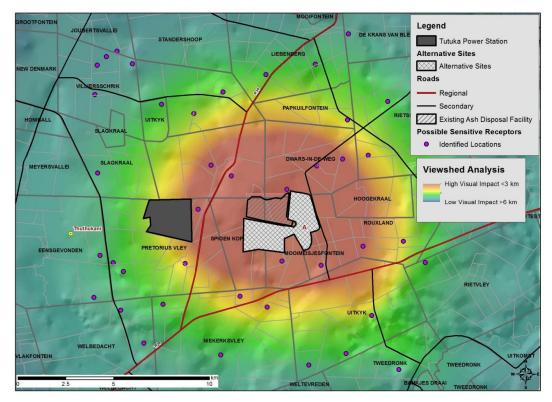
Figure 6: Typical proximity analysis for an ash disposal facility (Alternative A).
