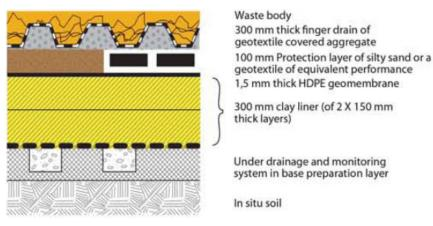
Figure 10.4: Class C Liner System
