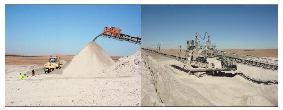
Figure 4.4: Stacker being used to dispose of ash at the Tutuka Power Station
