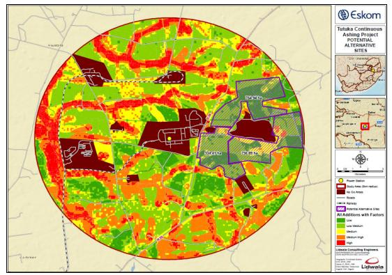
**Figure 7.5**: The potential areas, within the study area, large enough to accommodate the required area for the ash disposal facility (overlain on the sensitivity map).
