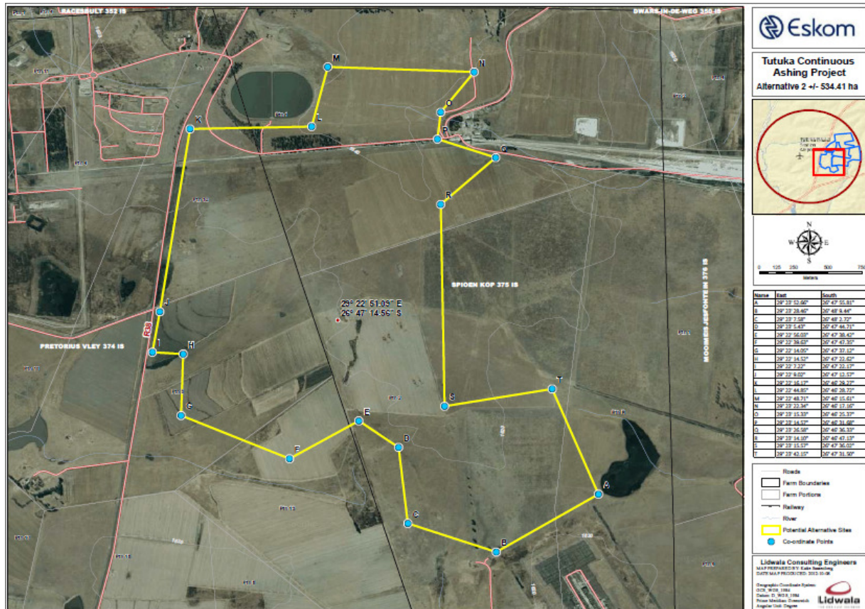
Figure 9.2. Proposed footprint (area) for the Tutuka Continuous Ash Disposal facility based on the findings of the EIA studies (Alternative C).
