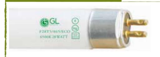
Figure 1 Fluorescent Lamp – F for Fluorescent, 28 for colour code, T5 for diameter, 28 Watt
