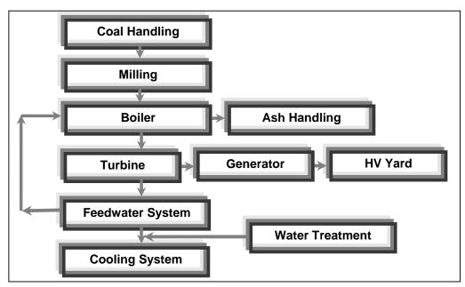
Figure 6: Process flow diagram of a typical coal fired power station
