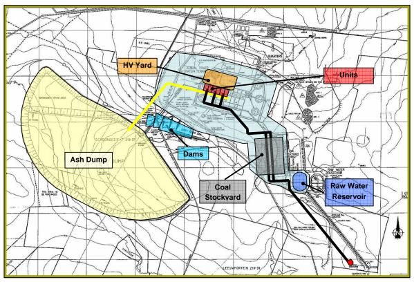
Figure 7: Typical power station layout
