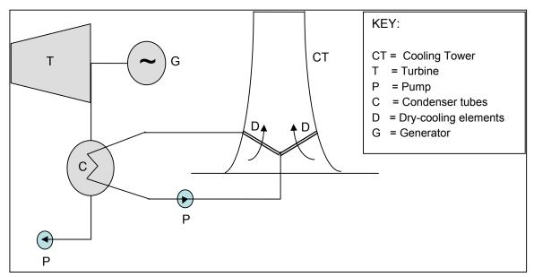
Figure 9: Indirect dry cooling
