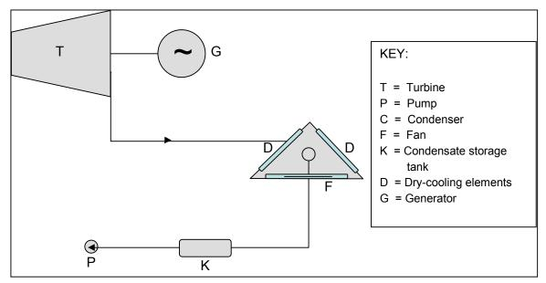
Figure 8: Direct dry cooling
