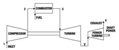
Figure 1: Schematic representation of a power generation gas turbine (Langston & Opdyke, Jr., 1997).
