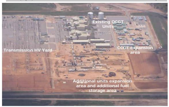
**Figure 3.1:** Aerial photograph of the Gourikwa Power Station site showing the existing power station infrastructure, the expansion site, as well as the areas for the placement of infrastructure associated with the proposed conversion
