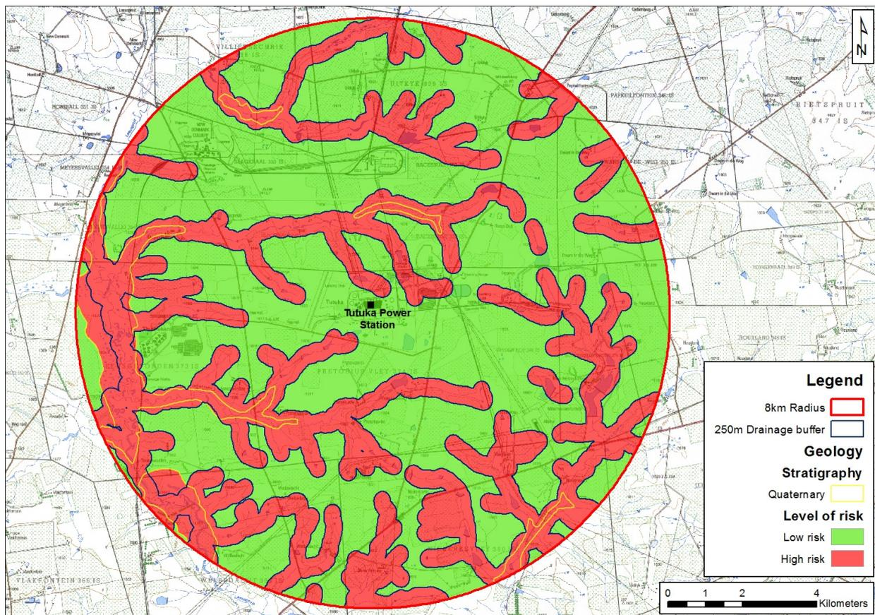
**FIGURE 6.3: PLAN IDENTIFYING LESS PREFERRED AND PREFERRED AREAS FOR THE PROPOSED EXTENSION TO THE ASH DISPOSAL FACILITIES AT TUTUKA POWER STATION**
