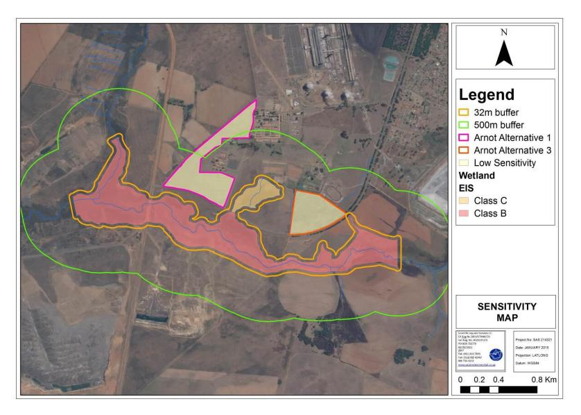
Figure 7: Wetland sensitivity mapping with associated buffers.
