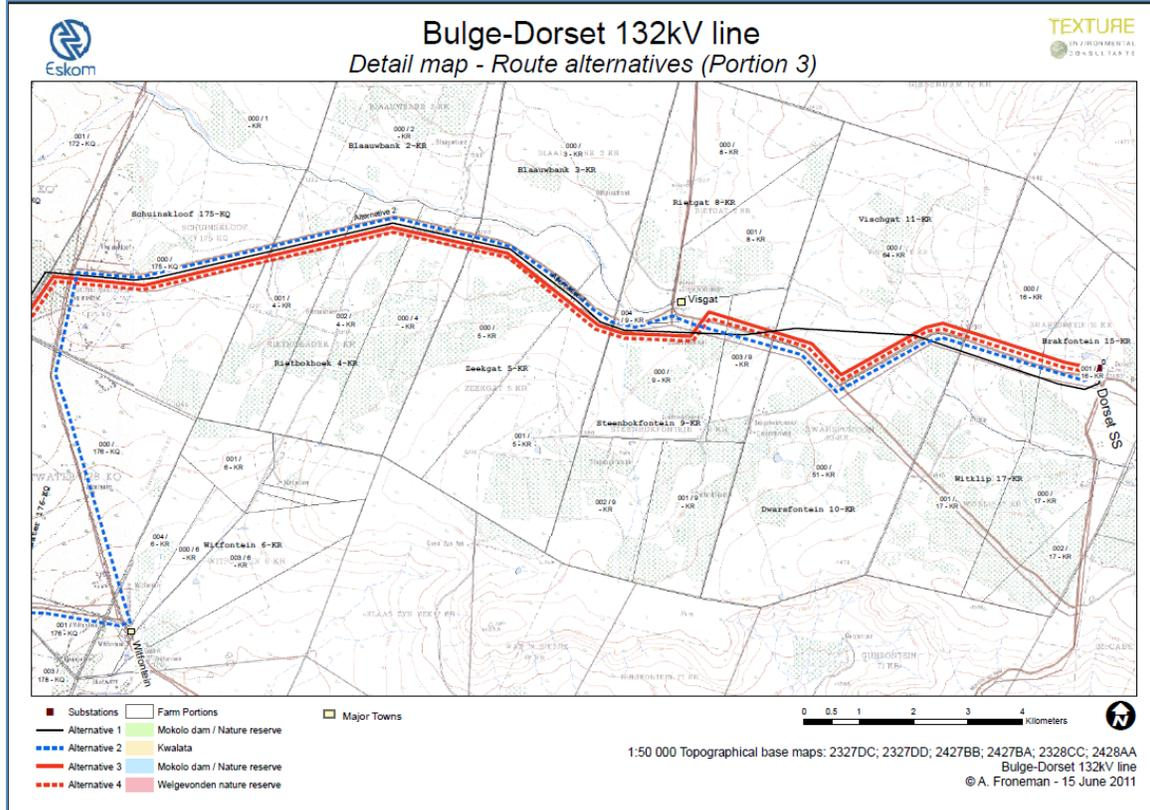
Figure 3: Portion 3 of the proposed alignments
