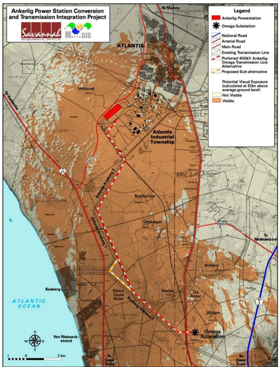
**Figure 6:** Potential visual exposure - transmission power line.
