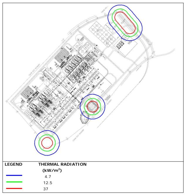
Figure 5-3 Thermal radiation from as a result of offloading operations
