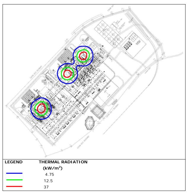
Figure 5-4 Thermal radiation from propane pool fires
