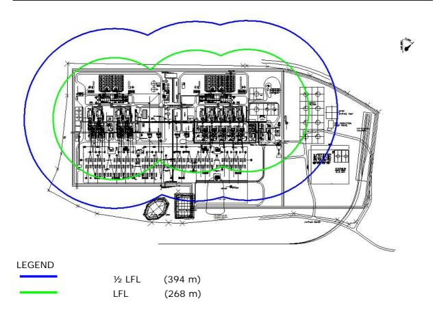
Figure 5-5 Maximum extent of the flammable cloud in the event of a catastrophic failure of the 20 m<sup>3</sup> delivery tanker
