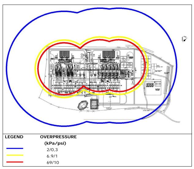
Figure 5-6 Worst case blast overpressure from a confined vapour cloud explosion from a catastrophic rupture of the 6.5 m<sup>3</sup> storage vessels
