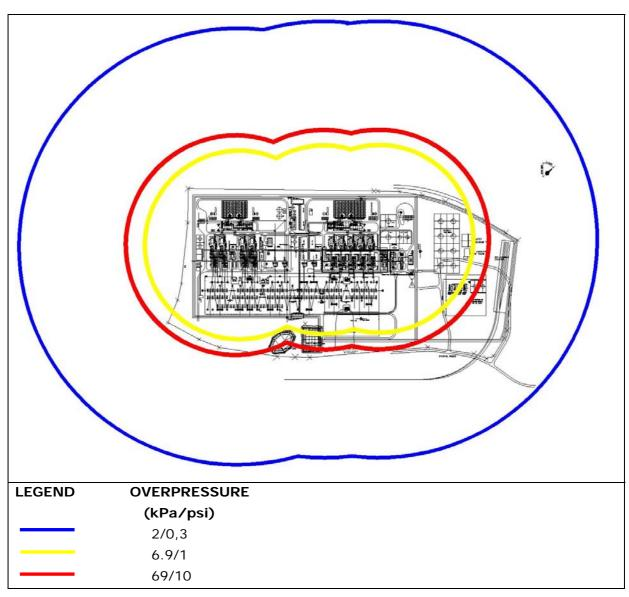
Figure 5-7 Worst case blast overpressure from a confined vapour cloud explosion from a catastrophic rupture of the 20 m<sup>3</sup> storage vessels
