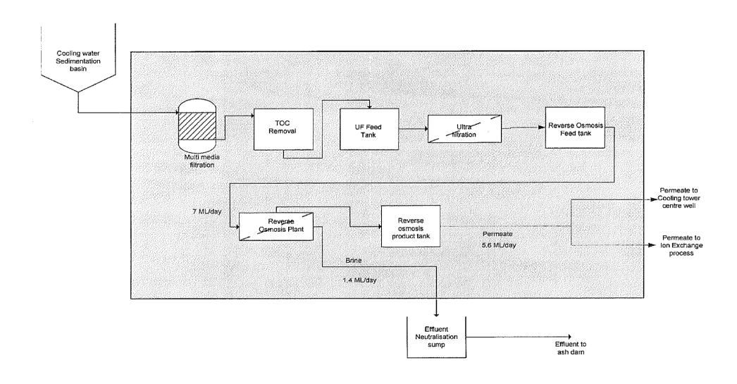
Figure 3: Flow diagram of proposed RO plant process (shaded grey) at Hendrina Power Station, Mpumalanga
