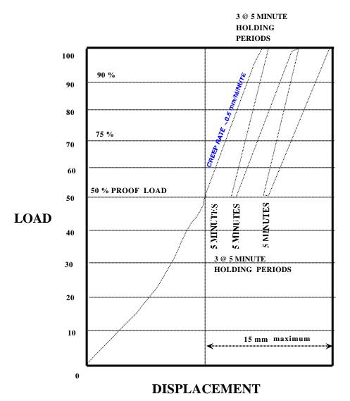
100 % Proof load = unfactored foundation reaction for critical loading condition
