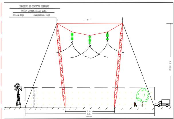
Figure 2: Cross-rope suspension tower structure
