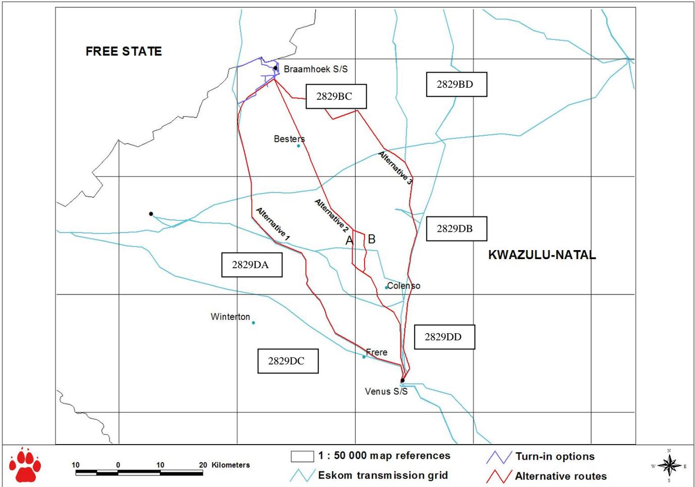
Figure 1: The study area for the Braamhoek – Venus 400 kV power line, showing the various routing options for this transmission power line, as well as the existing transmission grid.
