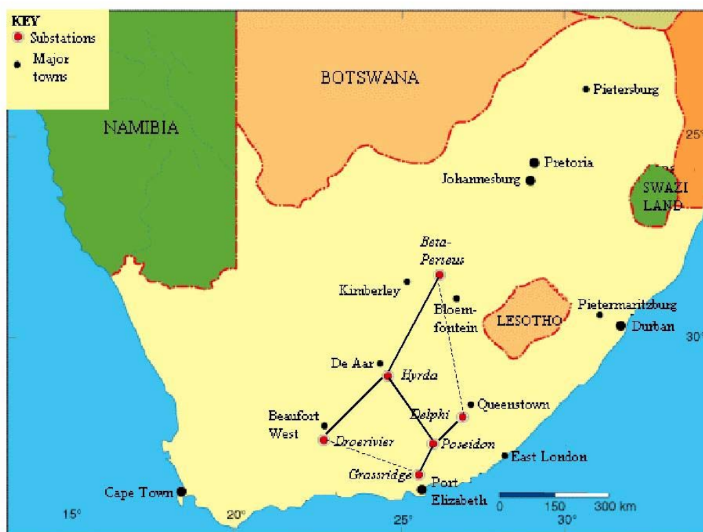
Figure 3.1: Schematic representation of the strengthening options for the Eskom Transmission network for the Greater Port Elizabeth area
