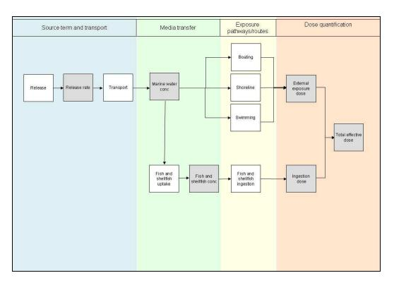
Figure 4.4: Pathway evaluation scheme for radionuclides discharged into the sea.
