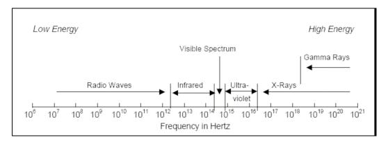
Figure 2.1: The electromagnetic spectrum.
