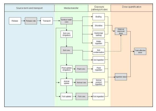
Figure 4.3: Pathway evaluation scheme for radionuclides discharged into surface water.
