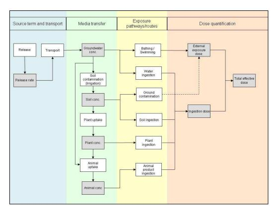
Figure 4.2: Pathway evaluation scheme for radionuclides discharged into groundwater.
