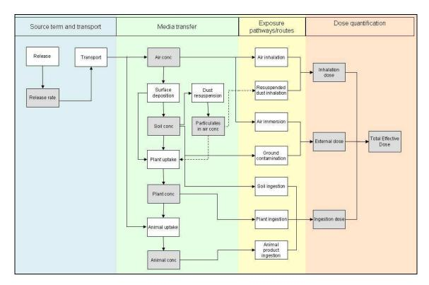
Figure 4.1: Pathway evaluation scheme for radionuclides discharged into air.
