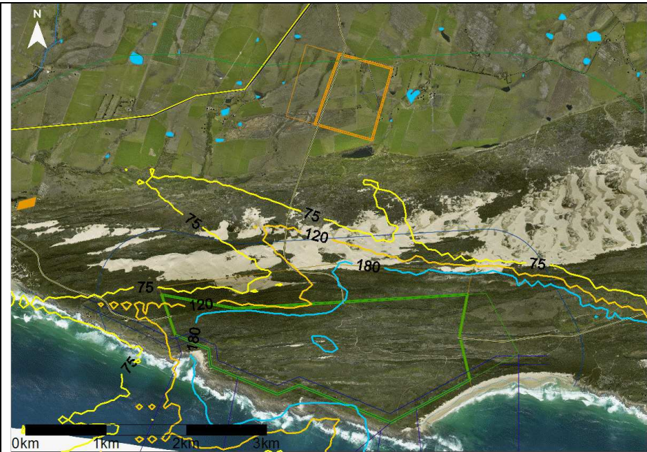
Figure 9-12: Predicted maximum daily average PM10 concentration levels during construction at Thyspunt with Road Option C and the envelope of the NPS on the east or west of the corridor (Unmitigated)
