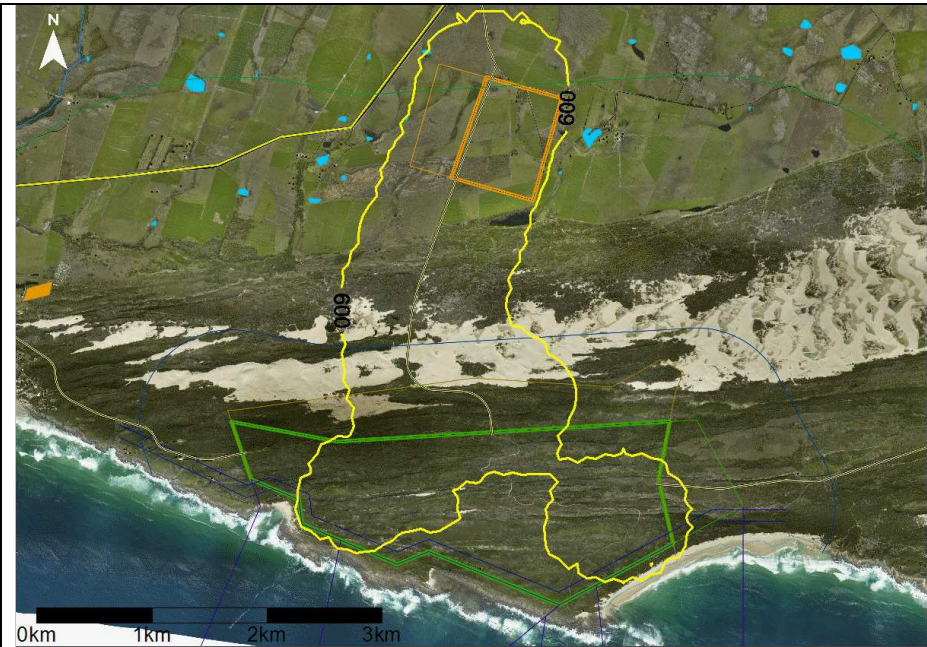
Figure 9-10: Predicted maximum daily average particle fallout rates ( \text{mg}/\text{m}^2/\text{day} ) during construction at Thyspunt with Road Option A and the envelope of the NPS on the east or west of the corridor (Unmitigated)
