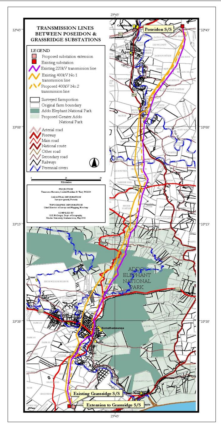
**Figure 1.1:** Map showing the existing and proposed Transmission lines between the Poseidon and Grassridge Substations, as well as the existing and proposed extension to Grassridge Substation
