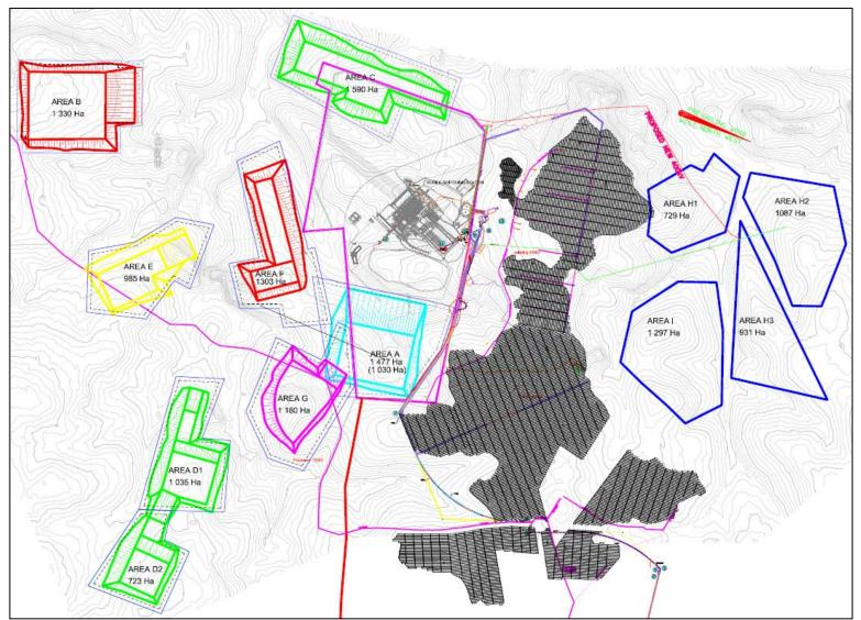
Figure 3-14: Models of sites west of power station. The model on Site A is designed to maximise storage capacity, therefore local infrastructure such as roads, pipelines and power lines will need to be deviated
