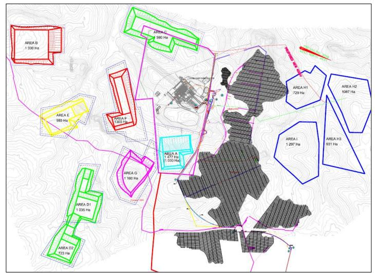
Figure 3-15: In this figure, a smaller model is designed on Site A to that take into account local infrastructure such as roads, pipelines and power lines as well as the river between Site A and the initial dump.
