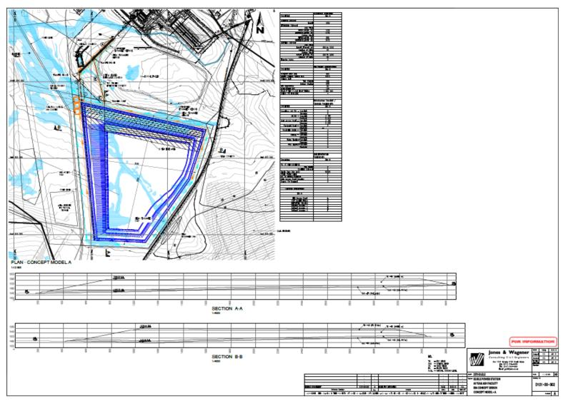
Figure 4.1 – Engineering Design – Site A (Ash Disposal Facility and Associated Conveyencing Infrastructure)
