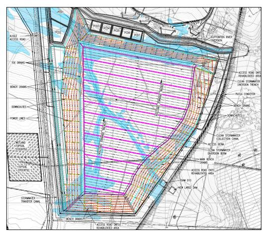
Figure 10: Stormwater infrastructure layout during rehabilitation
