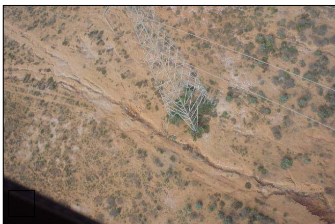
Figure 9 Aerial view of existing erosion of the access road near the Holgat River
