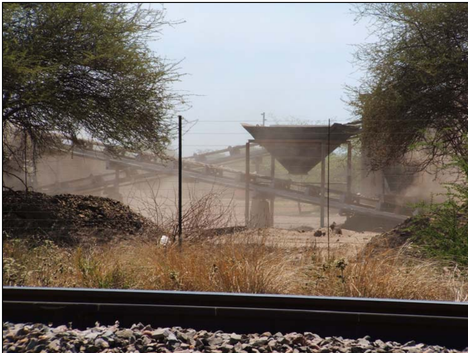
Figure 9.16: Fugitive emissions due to materials handling and raw material preparation at the brickmaking operations at Hanglip
