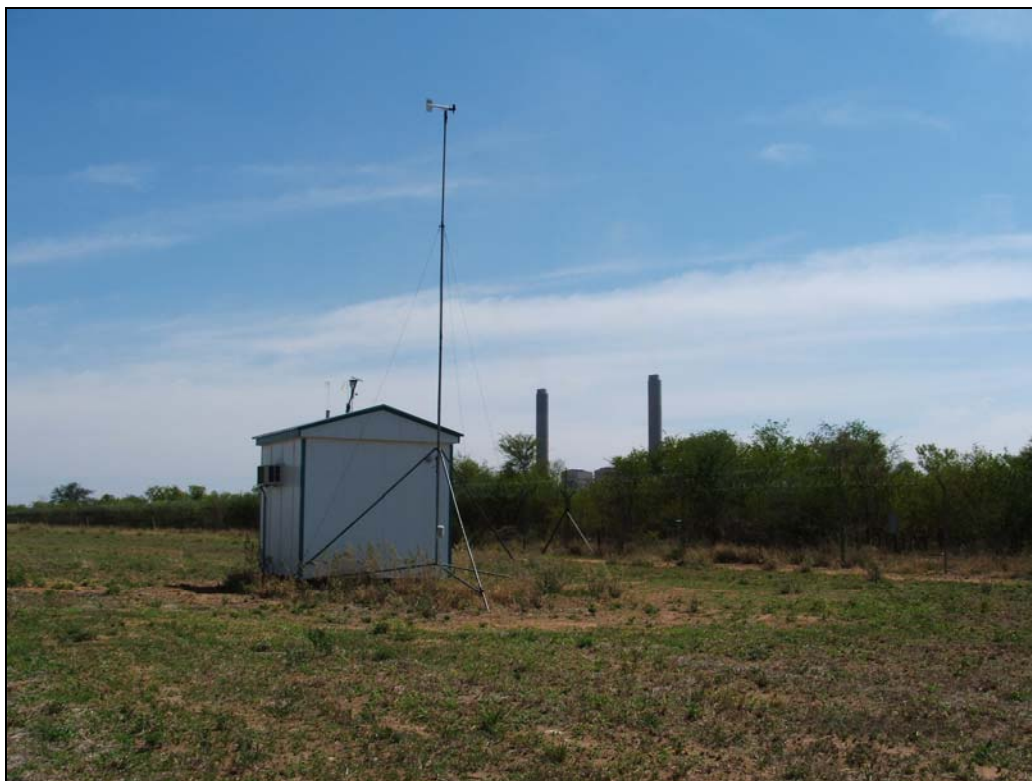
Figure 9.17 Grootstryd ambient air quality monitoring station located downwind of the Matimba Power Station.
