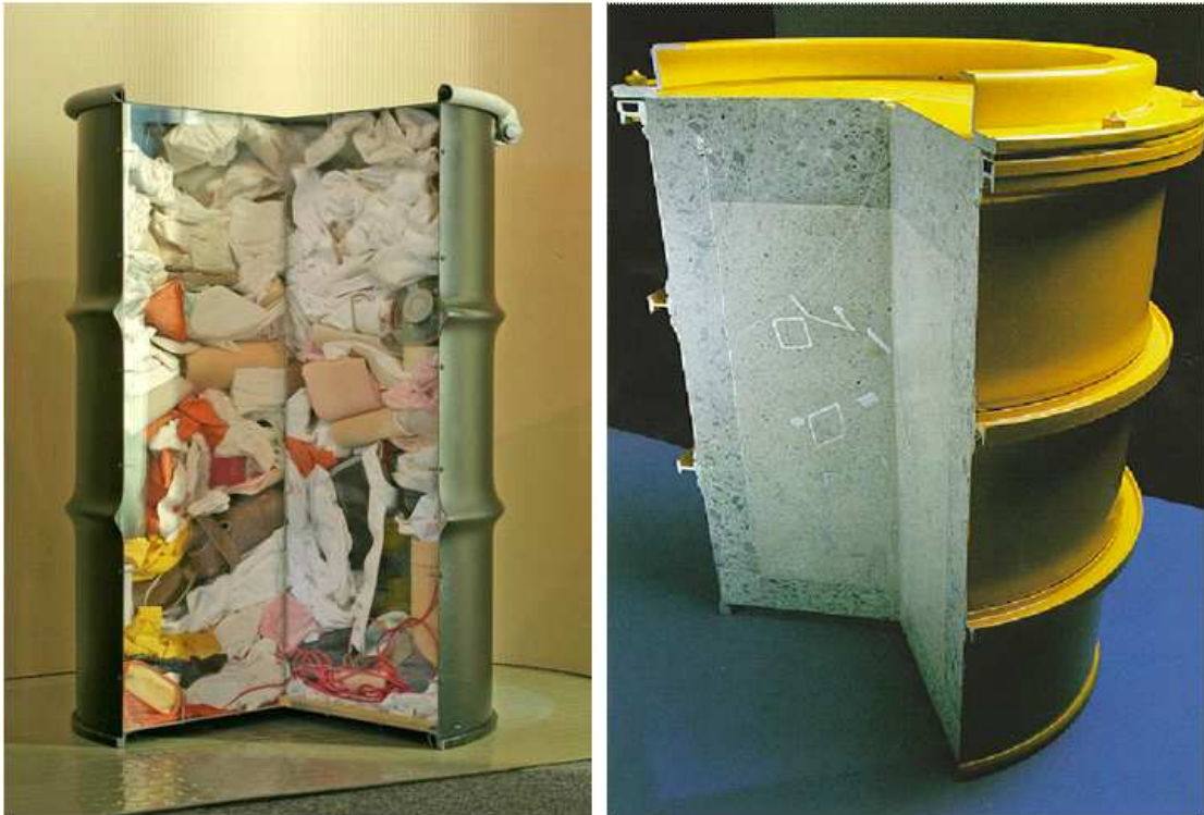
Figure 5.4 Examples of compactable LLW on the left and non-compactable ILW immobilised in cement on the right.
