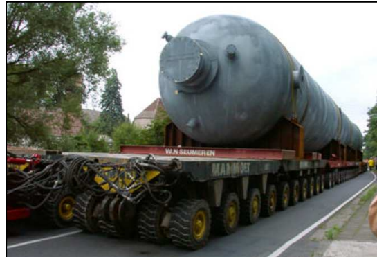
Figure 8.15: SPMT utilising the entire width of road 3
