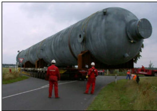
Figure 8.14: SPMT traversing an intersection 3
