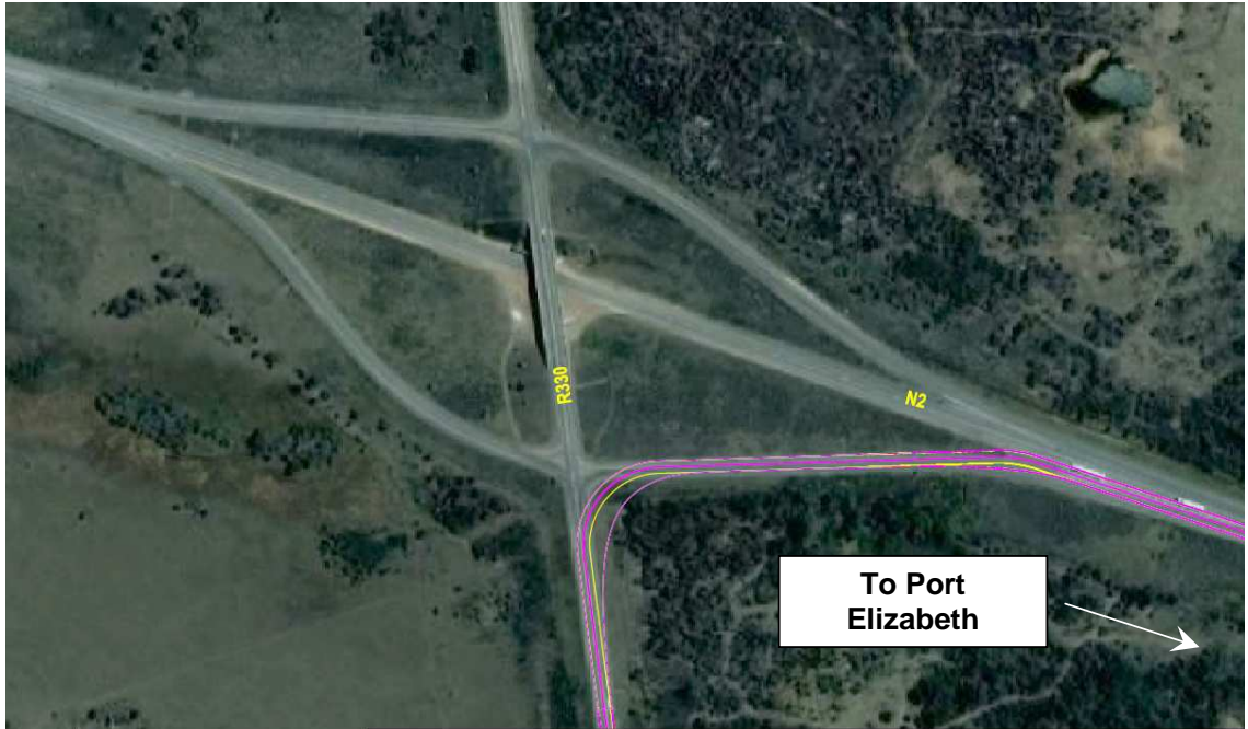
Figure 10.13 a: Abnormal load vehicle turning circle exiting N2 onto R330
