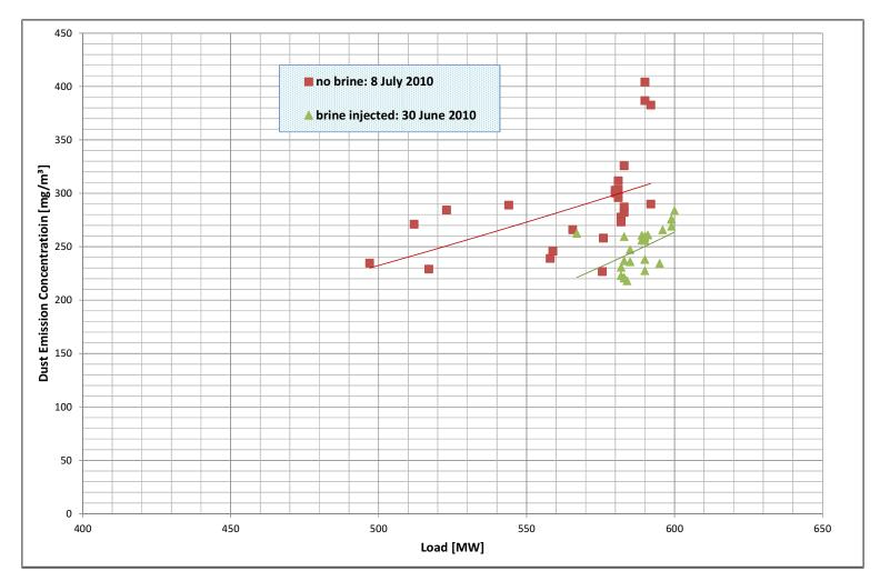
Figure 3-1: Comparison between the conditions with and without brine injection observe during the 24-hour monitoring campaign
