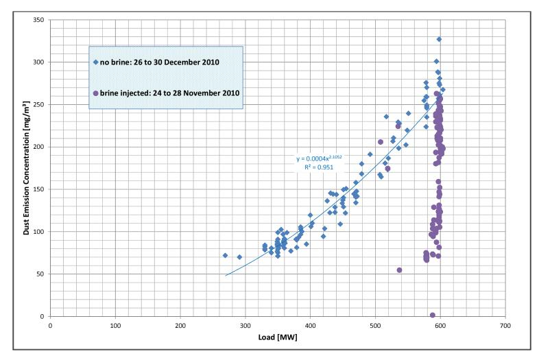
Figure 3-2: Comparison between the conditions with and without brine injection observe during the 5-day monitoring campaign
