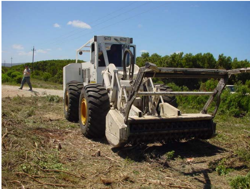
Figure 2. An example of a mechanical mulching machine.
