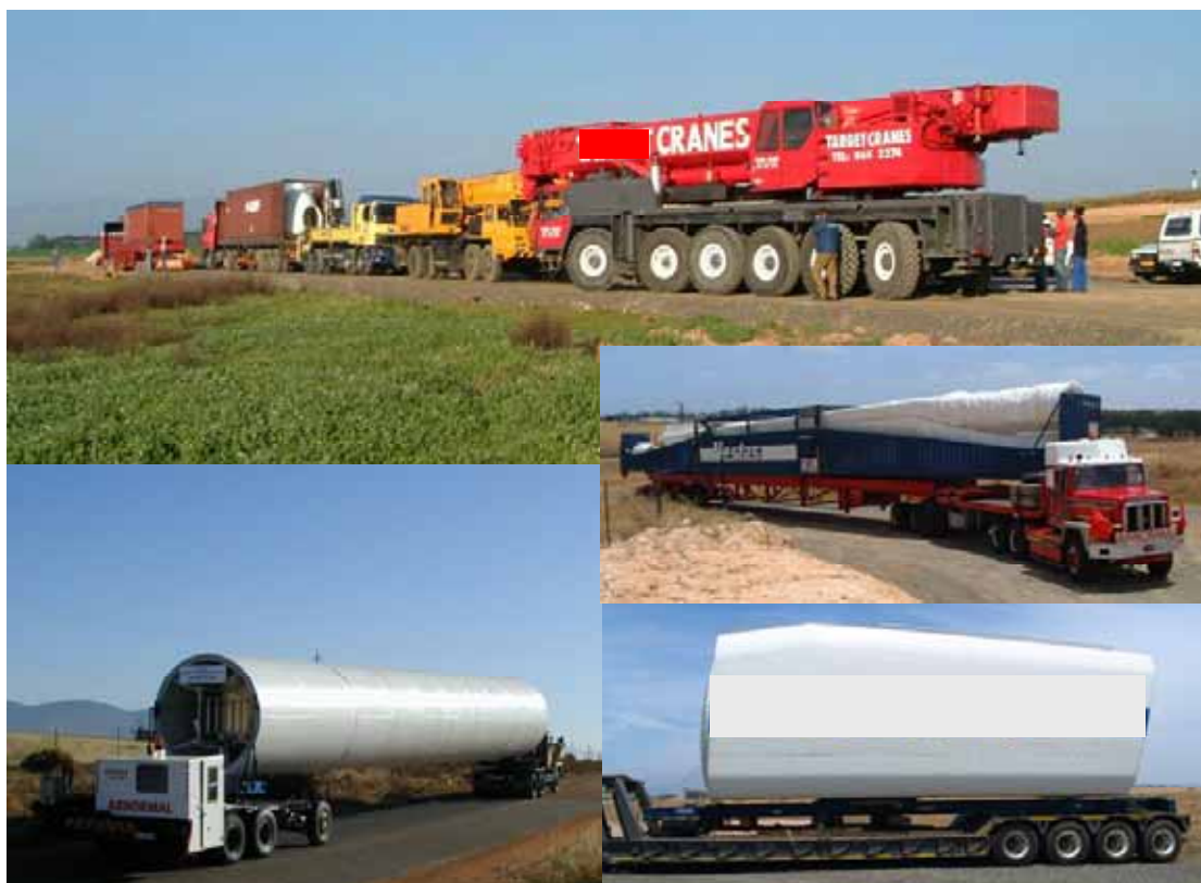
Figure 5.6: Photographs illustrating the equipment required for the transportation of turbine components to site (photographs courtesy of Eskom at during the construction of the Klipheuwel demonstration facility)
