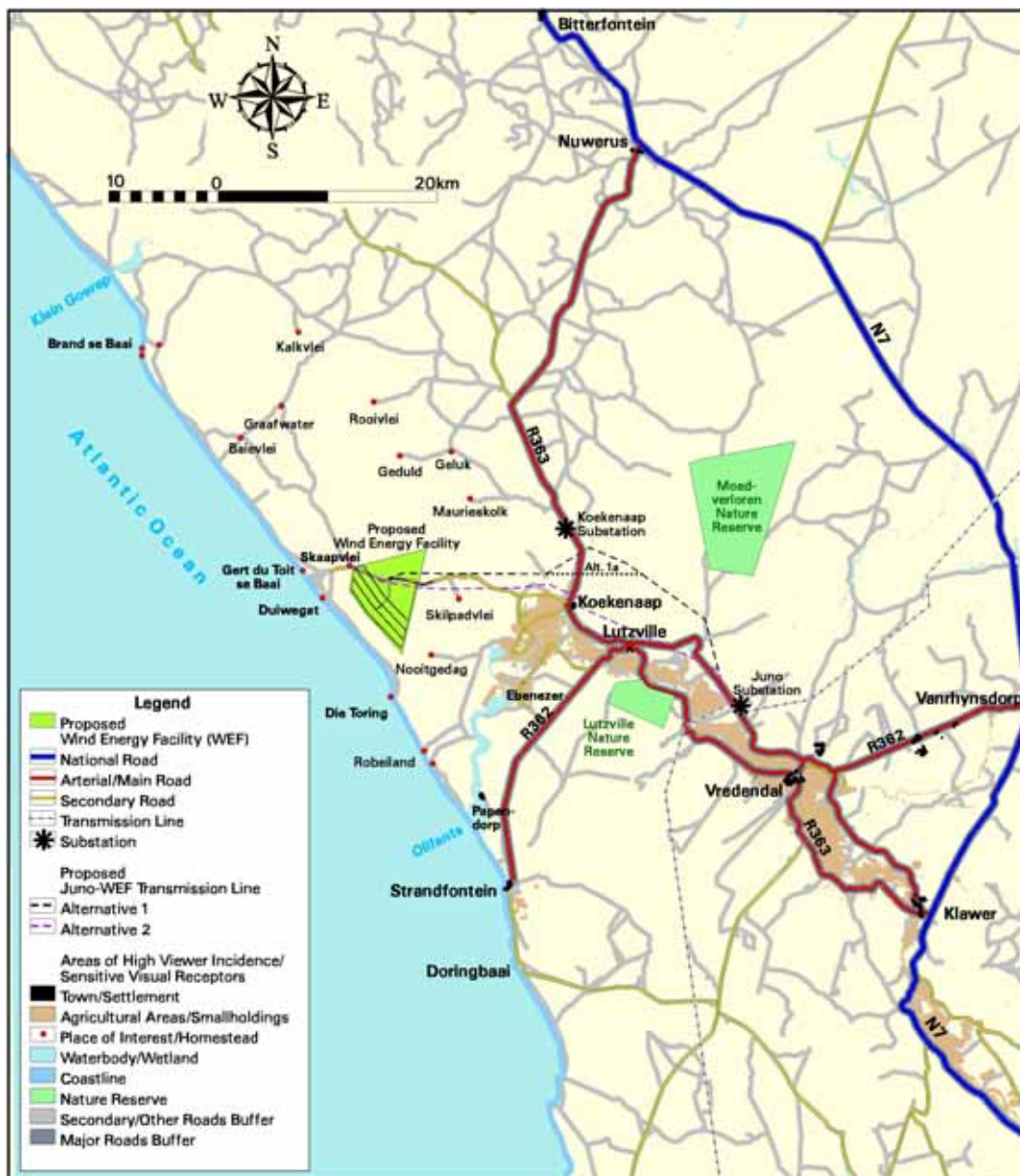
Figure 6.9: Locality map indicating the proposed wind energy facility site and proposed power line alternatives in relation to farm homesteads or residences and places of interest
