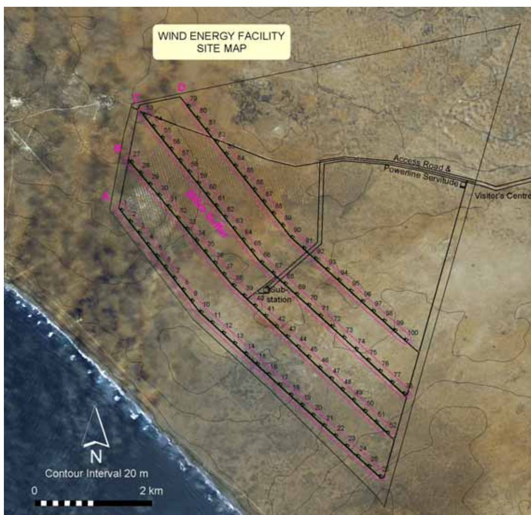
Figure 8.1: Illustration of the wind energy facility layout and the 200 m wide impact corridors identified for investigation.
