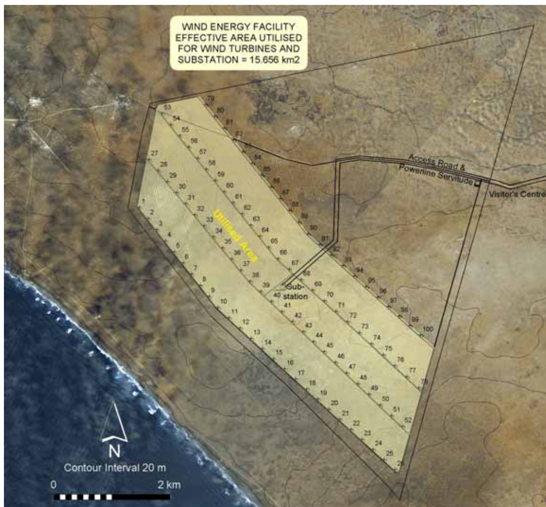
Figure 7.1: Illustration of the wind energy facility layout and the effective utilised area of 16 km 2 required to accommodate the bulk of the associated infrastructure.
