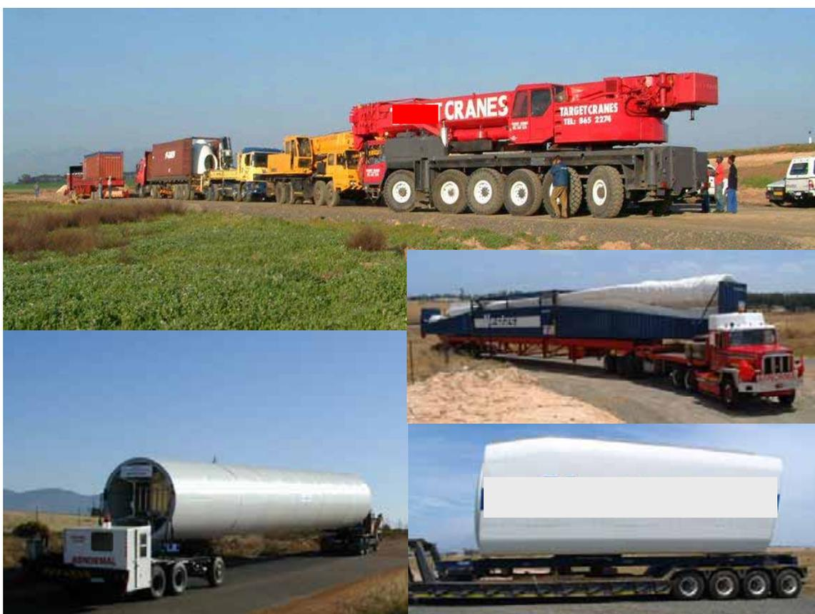
**Figure 7.5:** Photograph illustrating the equipment required for the transportation of turbine components to site (photographs courtesy of Eskom at during the construction of the Klipheuwel demonstration facility)
