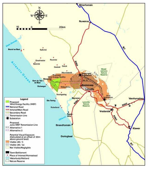
Figure 8.5: Potential visual exposure of the proposed power line Alternative 1 and 1a
