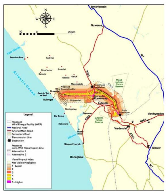
Figure 8.7: Visual impact index of the proposed power line Alternative 1 and Alternative 1a
