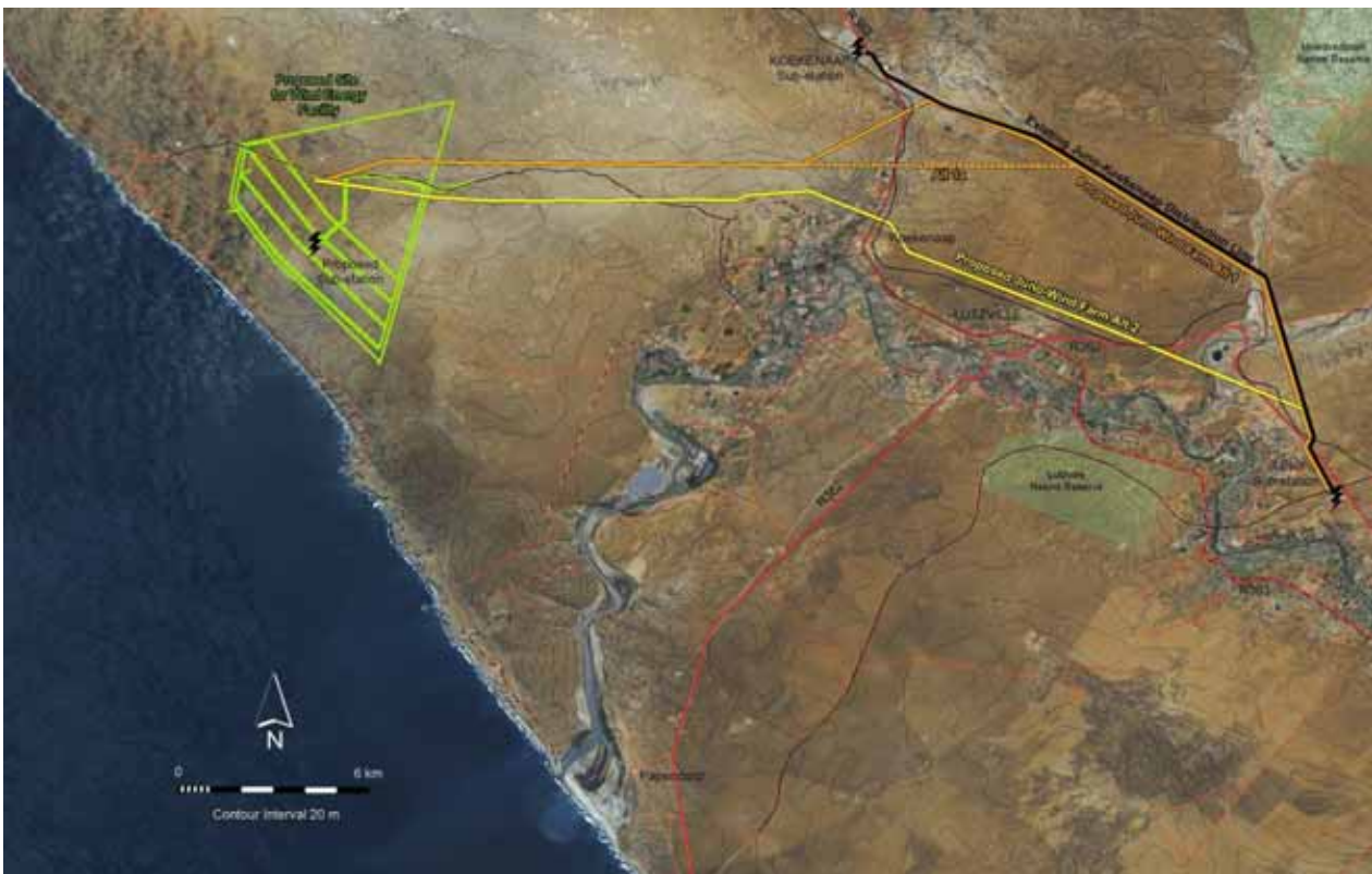
FIGURE 7. Expanded view of the WEF impact zone, indicating the two proposed 132 kV power line options connecting the facility to the Juno substation, and including sub-option 1a.
