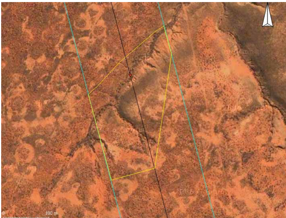
Figure 6. Erosion gully network indicated in yellow box. Note the extensive rilling present on the right hand slope of the drainage line. The erosion gullies could pose a threat to any tower located in this area. Upslope migration of eroded areas could potentially lead to undercutting of a tower.
