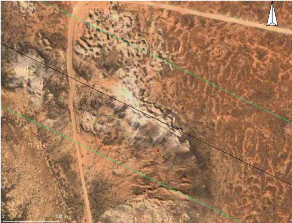
Figure 17. Steep slope subject to erosion and possible excavation. Towers located on the eroded slope would be exposed to a high erosion risk and hence should be excluded from consideration for this purpose.
