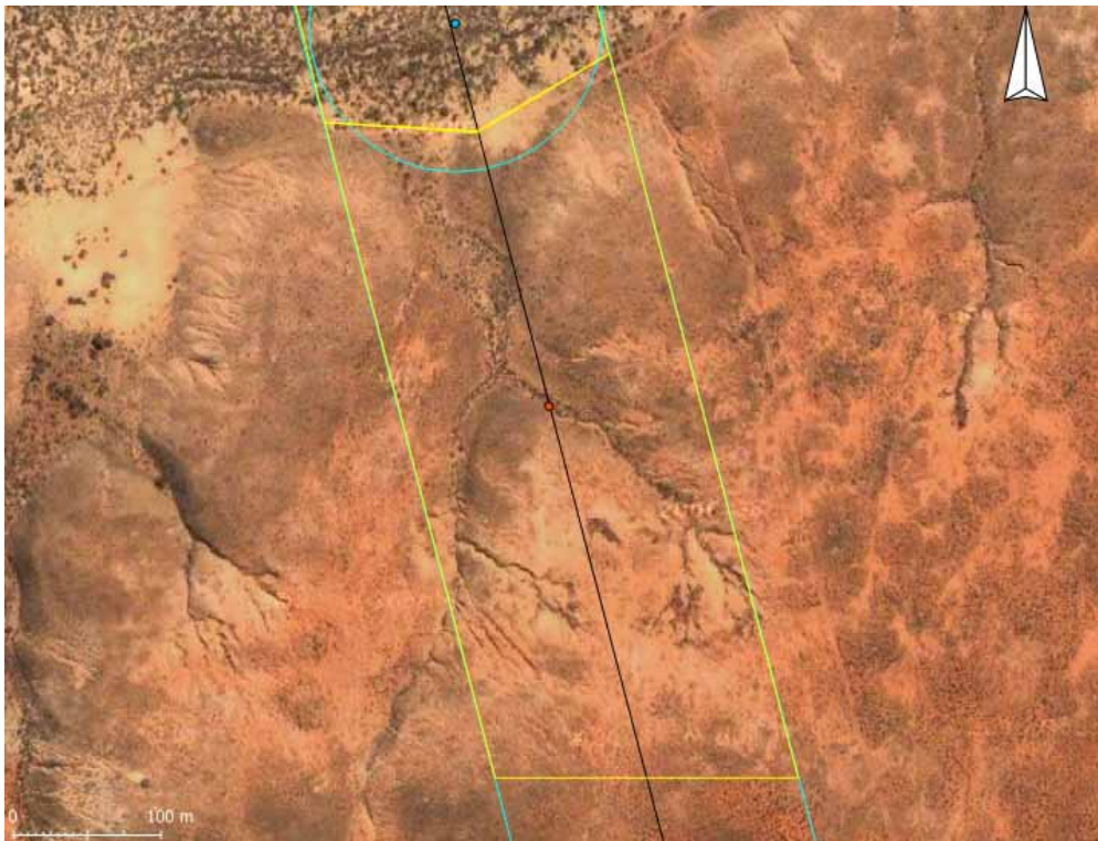
Figure 7. Erosion gully network. Most of the area highlighted in the yellow box is likely to be highly susceptible to sheet, rill or gully erosion. Towers located in this area could be undercut by the erosion. Runoff from roads could exacerbate erosion in the area.
