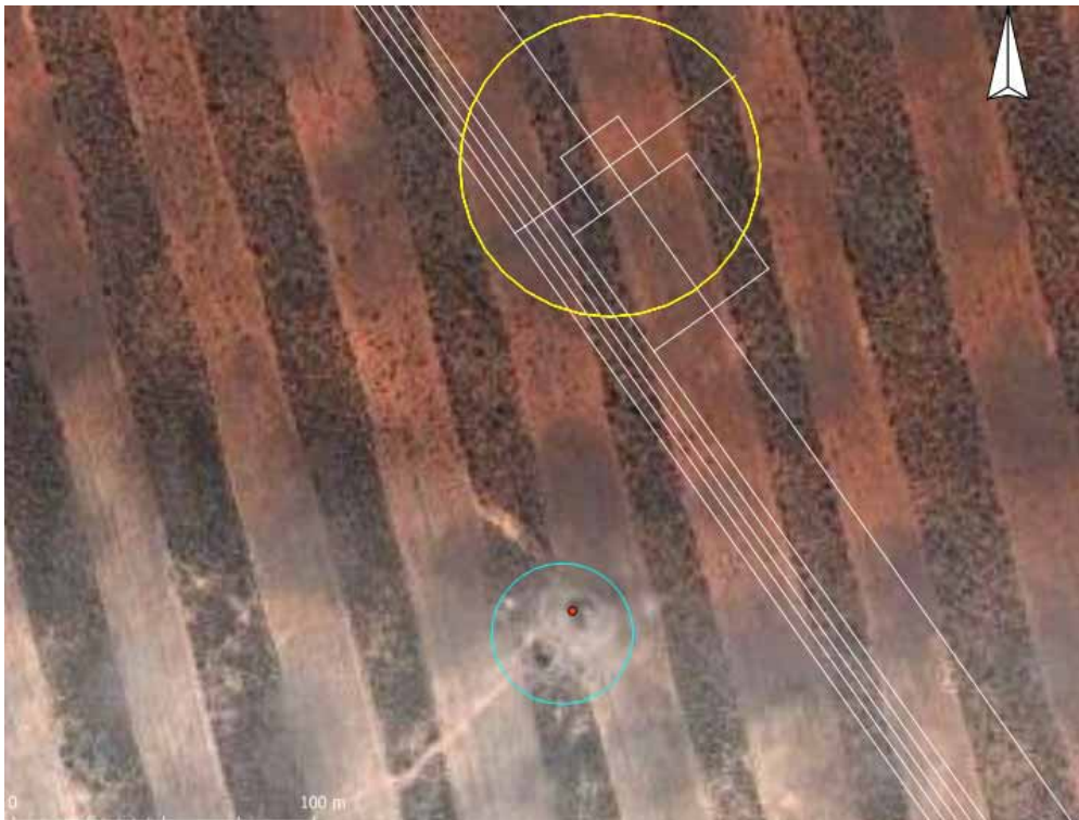
Figure 30. An area noted as a waterhole by Tim Hart (red dot). Most, if not all of the waterhole, is assumed to lie within the confines of the blue circle. The access road to the turbines will possibly have to be realigned slightly to remain outside the 50 m buffer around the wetland.
