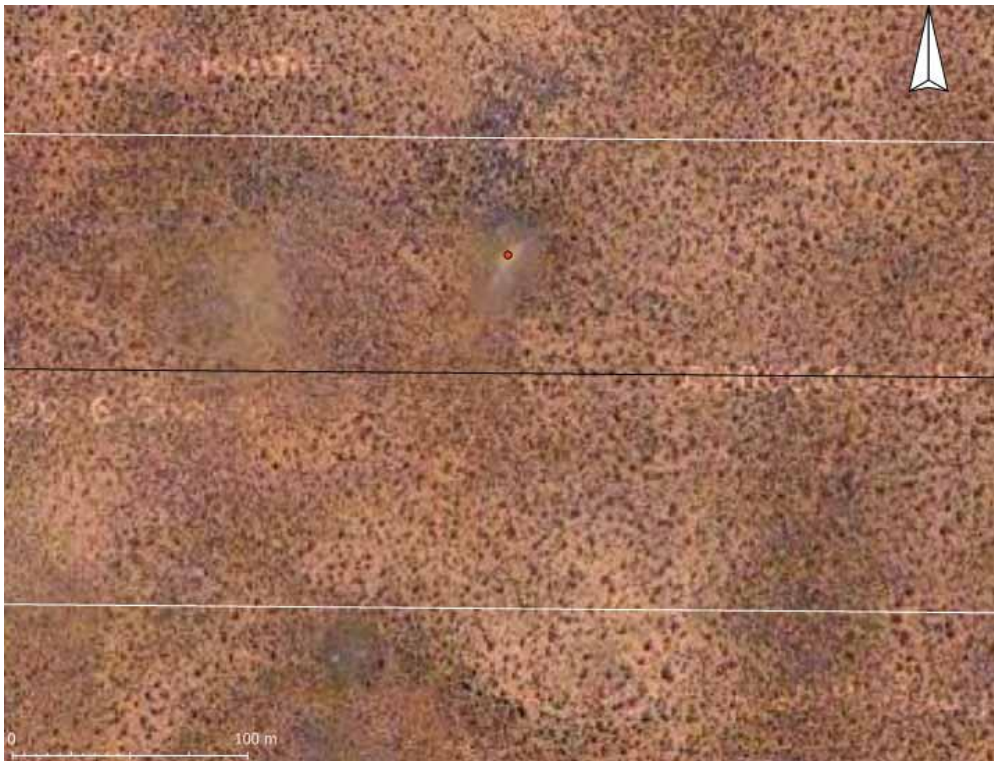
Figure 32. Enigmatic feature within the alternative 1a power line corridor. The feature may represent a pan, a blowout or another unknown feature. Even if the feature were to prove to be a pan, it would appear that it could easily be avoided for the siting of the towers or the access/maintenance road.
