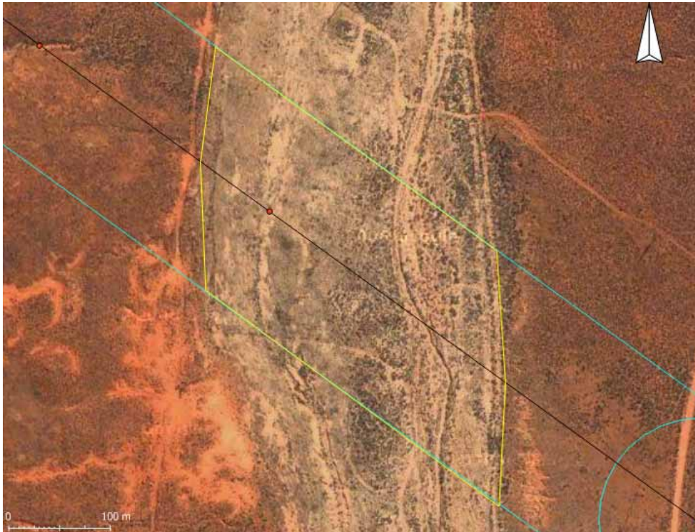
Figure 9. Broad floodplain of the Moedverloor River. If possible, towers should not be sited in the area demarcated with the yellow lines. Ideally, no roads should traverse these riparian corridors and associated floodplains. Maintenance roads should not result in unnecessary concentration of flows, which could lead to scouring and channel incision. Erosion in roadside ditches could also lead to upslope propagation of an erosion gully.
