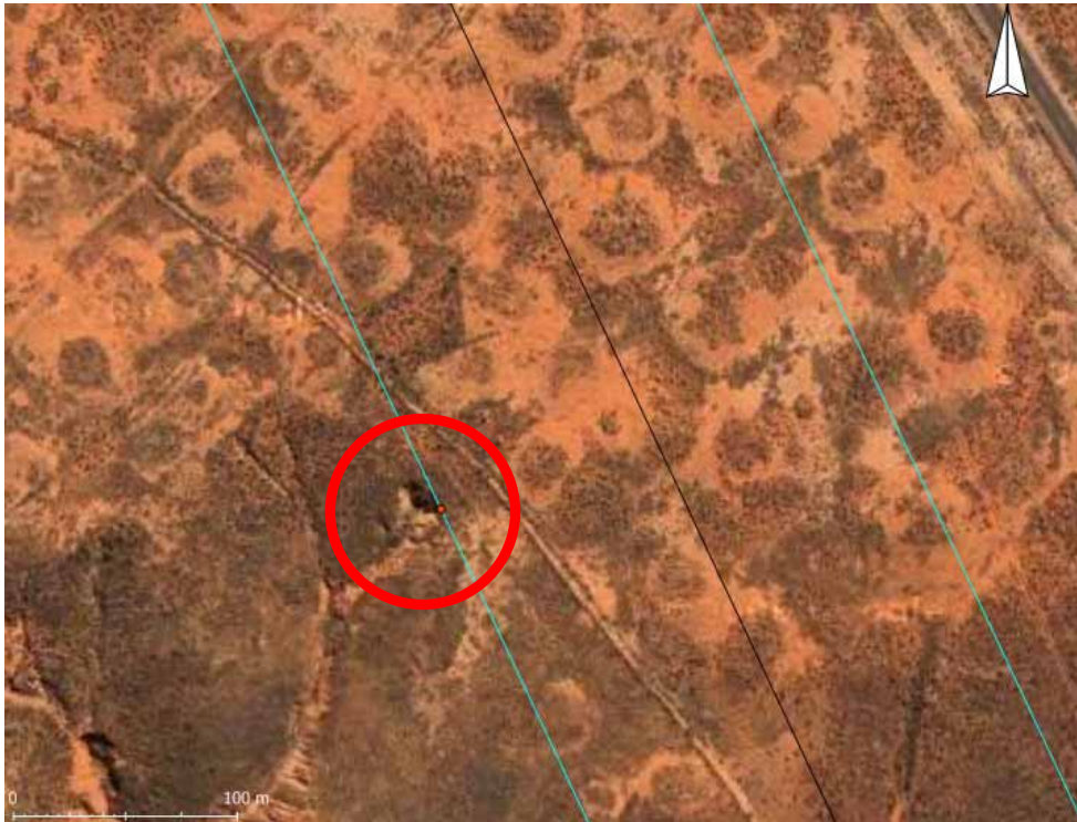
Figure 5. Gully head on the edge of the 200 m power line corridor. The headcut is expected to migrate further upslope and hence will pose a threat to any tower located in this area.
