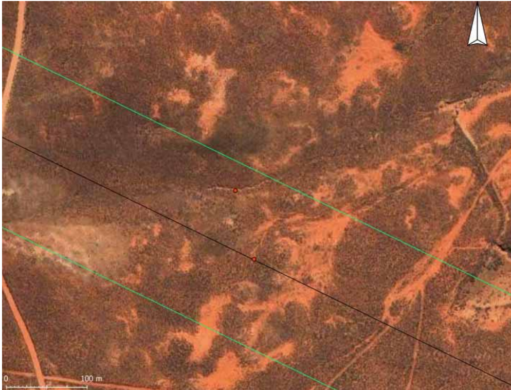
Figure 19. Incised drainage lines. Towers should not be located close to these features as fluvial erosion could result in the structures being undercut.
