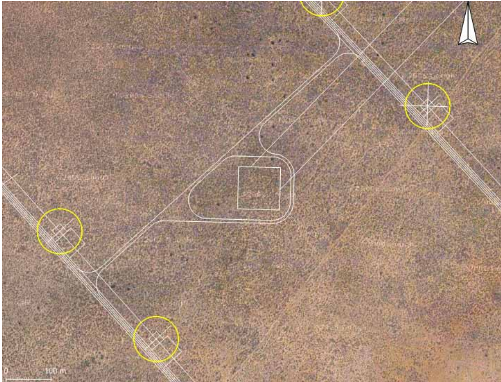
Figure 31. The area in the vicinity of the substation. Yellow circles indicate a distance of 50 m from a turbine. White square indicates the position of the substation in terms of the current layout. Note that it does not lie in close proximity to any sensitive area, with the obvious exception of the substrate, which is sensitive to wind erosion.
