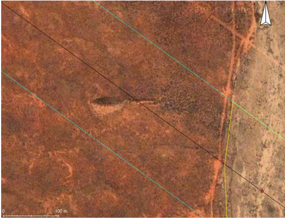
Figure 10. An incised channel segment. Towers should not be located close to this feature as fluvial erosion could result in the structure being undercut.
