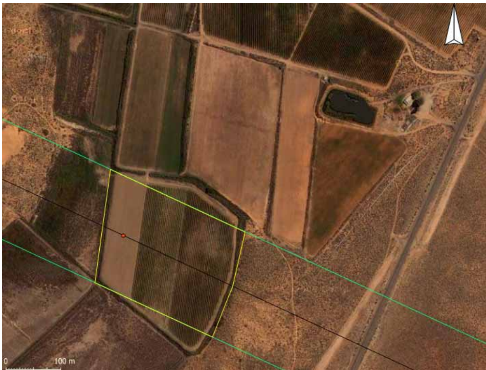
Figure 20. Modified floodplain of the Jaagleegte River. If possible, towers should not be sited in the area demarcated with the yellow lines. Maintenance roads should not result in unnecessary concentration of flows, which could lead to scouring and channel incision.
