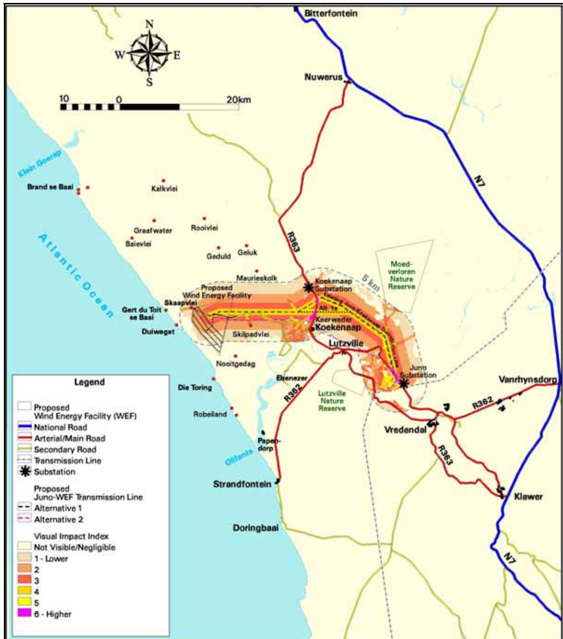
Figure 12: Visual impact index of the proposed transmission line Alternative 1
