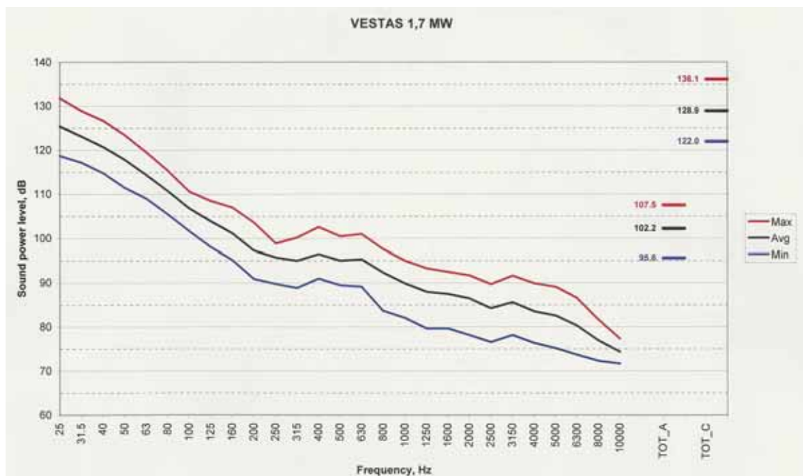
FIGURE 6 Sound power level emission of a Vestas, V66 wind turbine
