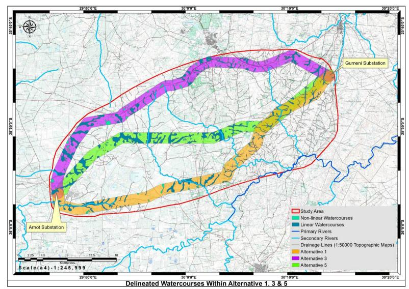
**Figure 4:** Delineated watercourses based on onscreen digitising within each alternative corridor. Watercourses were demarcated as Linear and Non-linear features and include a range of watercourse types such as wetlands, dams, riparian habitat, natural channels and indistinct headwater drainage lines.
