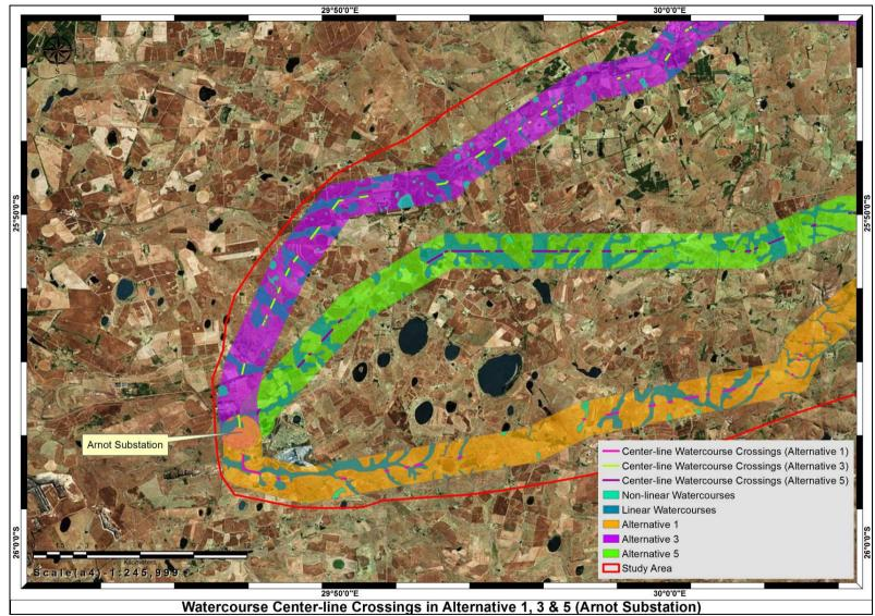
Figure 5: Demarcated watercourses within the three alternative corridors and watercourse crossings along the center-line of each alternative in the western study area section.
