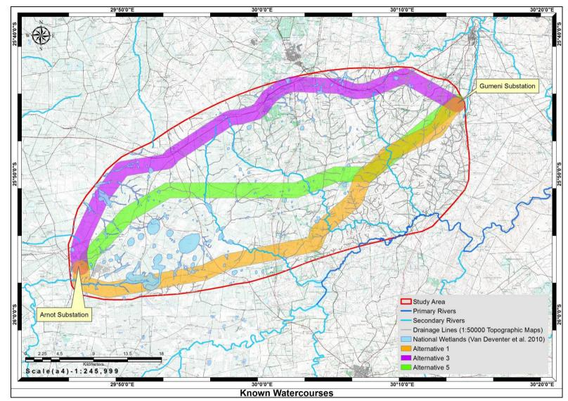
Figure 3: Known wetlands and other watercourses within the Arnot-Gumeni study area and alternatives based on existing spatial datasets; primary and secondary rivers from Middleton & Bailey (2008).
