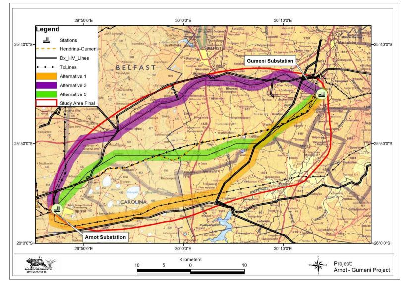
Figure 1: Illustrates the study area, main roads, start point (Arnot Substation) and endpoint (Gumeni Substation), as well as the three route alternative corridors (1, 3 & 5).
