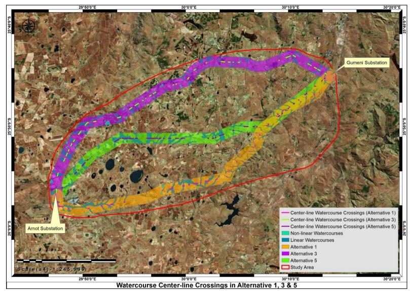
Figure 7: Watercourse crossings along the center-line of each alternative.
