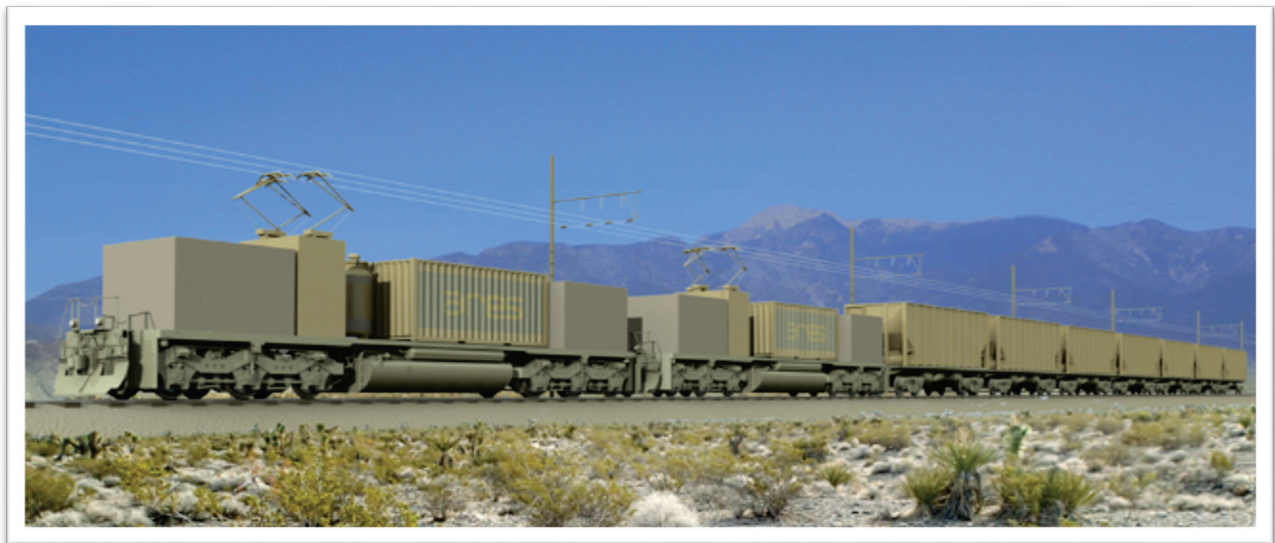
Artists concept for a 50-MW/12.5-MWh gravity-based potential energy storage system
