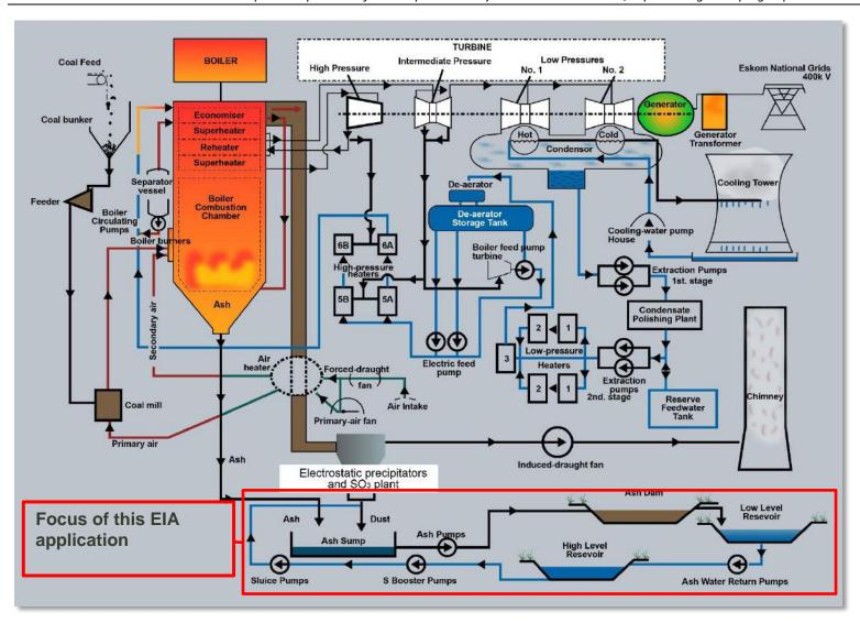
Figure 3-3 | Flow chart of the operation showing inputs and outputs of the process at Kriel Power Station (including the Ash Disposal Facility in red)
