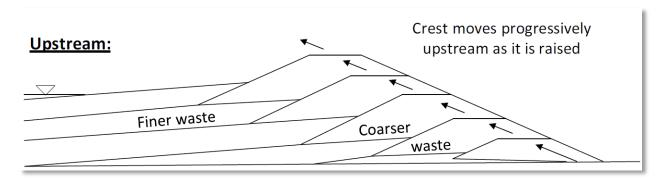
Figure 3-7 | Upstream development of ash dam (Chamber of mines, 1996)
