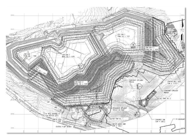
**Figure 3-6** | Ash Dam 4 Concept 2016 preferred alternative, consisting of only AD 4.1 and 4.2 (Jones & Wagener, 2016)
