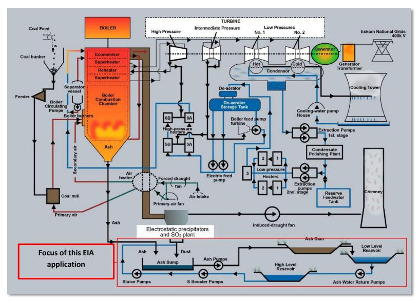
Figure 1: Flow chart of the operation showing all inputs and outputs of the process at Kriel Power Station which includes the Ash Disposal Facility
