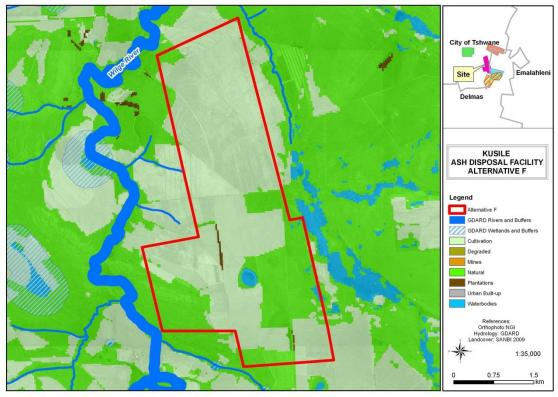
Figure 15: Orthophoto of the 1303 hectares Area F. Note its proximity to the Wilge River, the pan and the wetland outside its eastern boundary. GDARC Rivers and Buffers (dark blue) and Waterbodies (bright blue) mapped, are deemed as sensitive.
