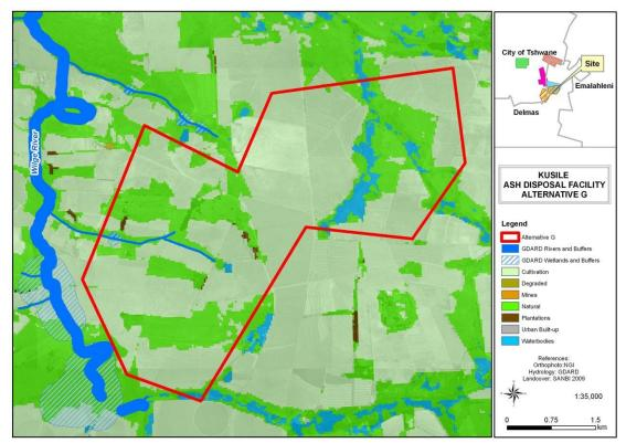
Figure 13: Orthophoto of 1857 ha Scenario 4 (Area G1 and G2). Note its proximity to the Wilge River and a wetland to its southern boundary. GDARC Rivers and Buffers (dark blue) and Waterbodies (bright blue) mapped, are deemed as sensitive.
