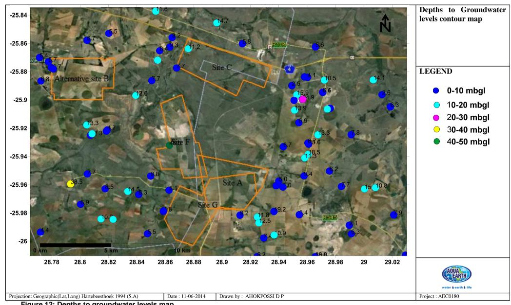
Figure 12: Depths to groundwater levels map
