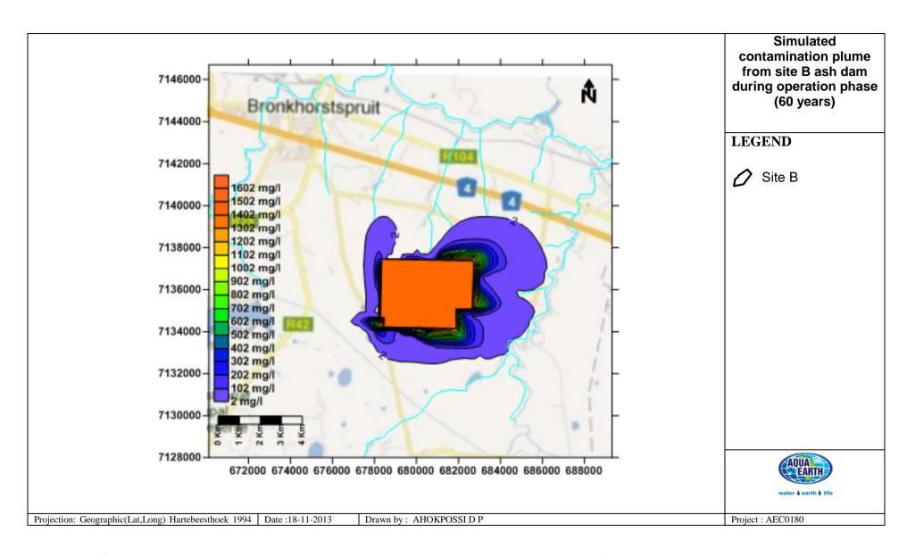
Figure 62: Simulated contamination plume from Alternative B ADF during operation phase (60 years)
