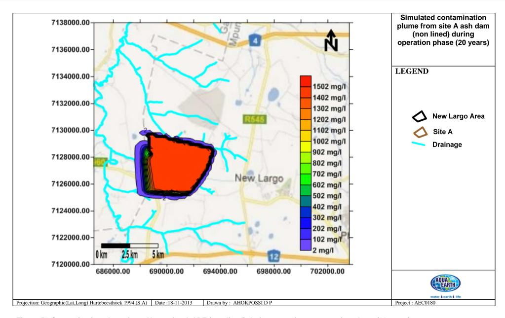
Figure 57:Contamination plume from Alternative A ADF (non lined) during operation-construction phase (20 years)
