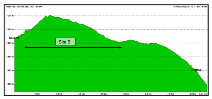
Figure 55: West-East (KABH42-KABH62) cross section over the preferred site B
