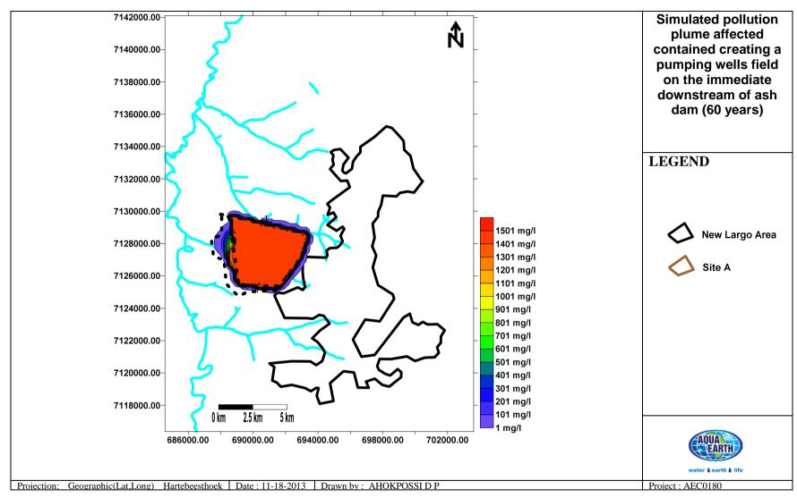
Figure 71: Simulated pollution plume contained by a pumping wells field on the immediate downstream of ADF (60 years
