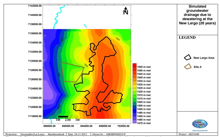
Figure 65: Simulated groundwater drainage due to dewatering at the New Largo (20 years)
