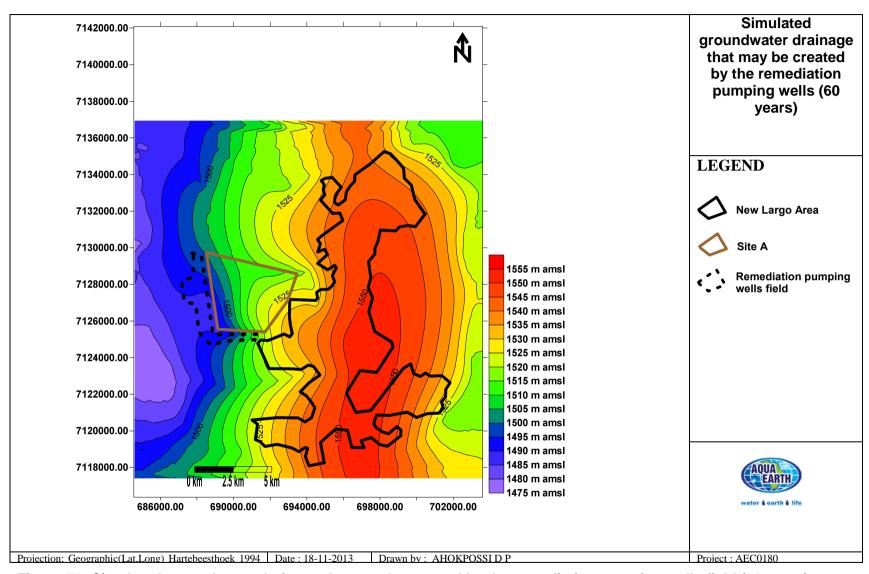
Figure 70: Simulated groundwater drainage that may be created by the remediation pumping wells field (60 years)
